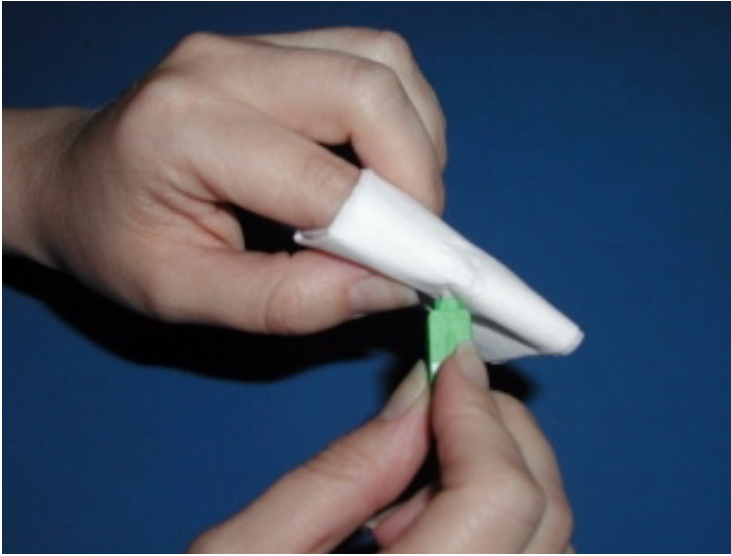
Figure 19 Wiping the connector with a Kim wiper
